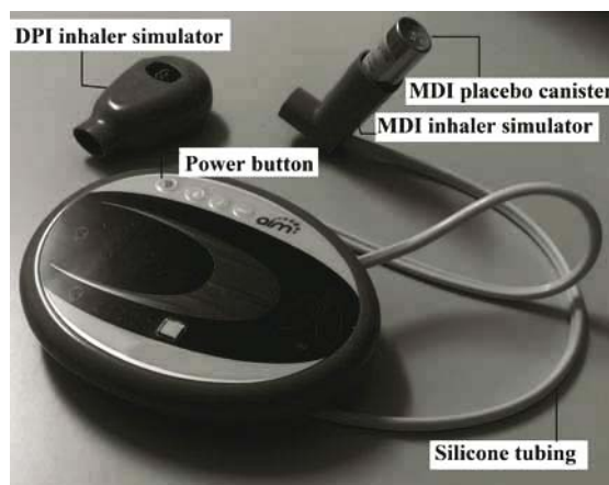
Figure 1. Main components of the AIM devices
