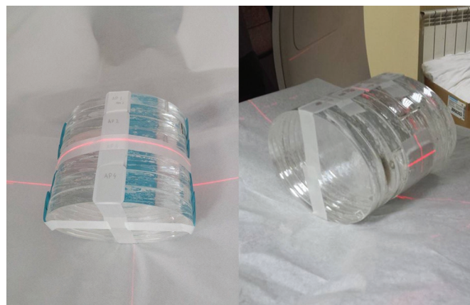
Figure 1. Positioning of the films along the ellipsoid PMMA phantom a) CT Unit A, b) CT unit C
